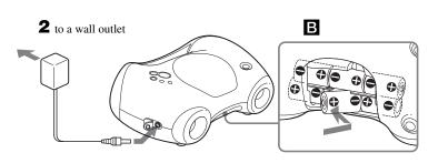
Connect the AC power adaptor A or insert six size D (R20) batteries (not supplied) into the battery compartment B.
